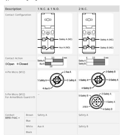
$<sup>\</sup>star$  Replace symbol with 2 (2 m), 5 (5 m) or 10 (10 m) for standard cable lengths.
